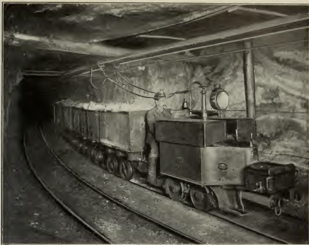
FIG. 25. ELECTRIC MINE LOCOMOTIVE, NEUSTASSFÜRT ROCK-SALT MINES.
